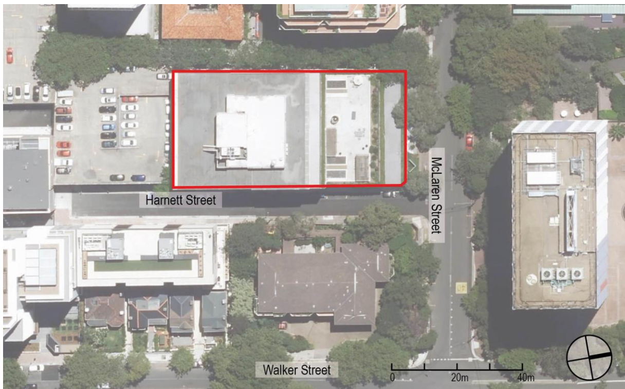
Figure 1.2 Site plan showing the layout of 41 McLaren Street (bounded by the red outline) and the staggered massing of the blocks comprising Simsmetal House, the associated rooftop terraces and plant-room on the southernmost roof. (Source: SIX Maps with GML additions, 2017)
